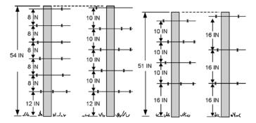
Figure 2. Common wire spacings for barbed wire fences.
