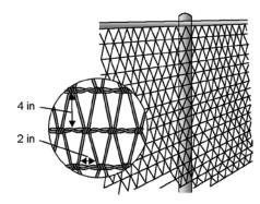
Figure 4. Detail of a diamond-mesh fence.
