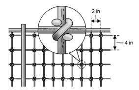
Figure 3. Detail of a square knot-mesh fence.
