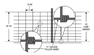
Figure 1. Design numbers assigned to woven wire fences (e.g. "1047 - 12 - 11") indicate the number of line wires (10), height (47 in), stay wire spacing (12 in), and filler wire size (11 gauge).
